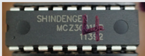
Microchip PIC16f1827 microcontrollers fraudulently re-labelled as Shindengen MCZ3001DB microcontrollers
