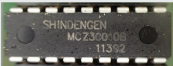
Microchip PIC16f1827 microcontrollers fraudulently re-labelled as Shindengen MCZ3001DB microcontrollers
