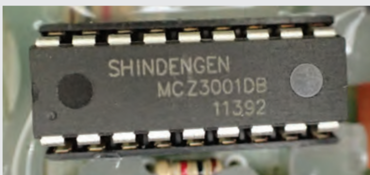
A Microchip PIC16f1827 microcontroller fraudulently re-labelled as a Shindengen MCZ3001DB microcontroller
